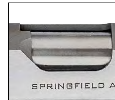
LOWERED & FLARED EJECTION PORT
