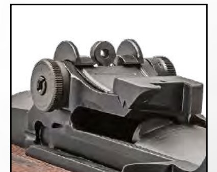
MILITARY APERTURE .069", ADJUSTABLE FOR BOTH WINDAGE & ELEVATION
