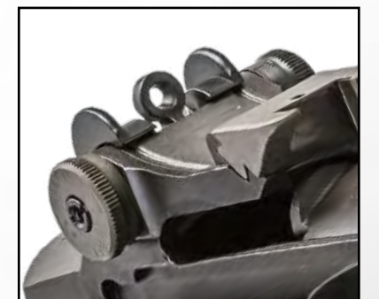
ENLARGED MILITARY APERTURE .135 WITH MOA ADJ FOR BOTH WINDAGE & ELEVATION
