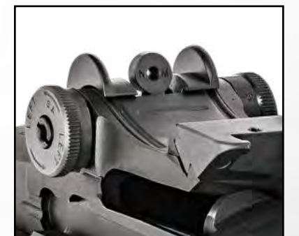
MATCH-GRADE NON-HOODED .0520 APERTURE, 1/2 MOA ADJ FOR WINDAGE & MOA FOR ELEVATION
